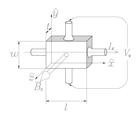
When steady state is reached, there will be no net flow of charge in the y direction, since the electrical and magnetic forces on the charge carriers in that direction must be balanced. Since the force of an electric field on a charge q is  $q\mathbf{E}$ , we have
