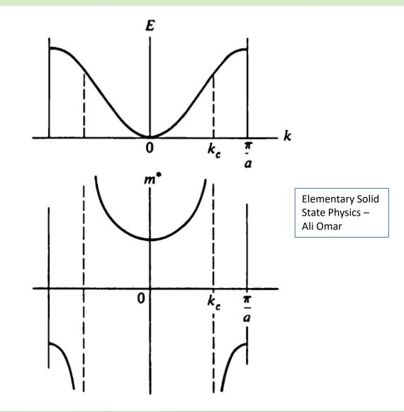
The effective mass  $m^*$  is positive near the bottom of the band, where the curvature is positive. But near the top, where the band curvature is negative, the effective mass is also negative.
