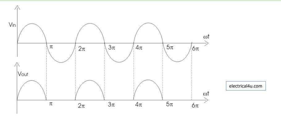
Ripple is the unwanted AC component remaining when converting the AC voltage waveform into a DC waveform. Even though we try out best to remove all AC components, there is still some small amount left on the output side which pulsates the DC waveform. This undesirable AC component is called ripple.
