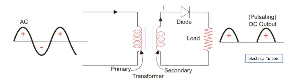
$$V_0(t) = \begin{cases} V_m \sin(\omega t), & 0 \le t \le T/2 \\ 0, & T/2 \le t \le T \end{cases}$$
