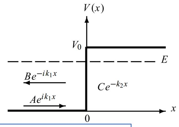
$$J_{transmitted} = \frac{\hbar}{2im} \left( \psi_t(x) \frac{d\psi_t(x)}{dx} - \psi_t(x) \frac{d\psi_t(x)}{dx} \right) = 0.$$
