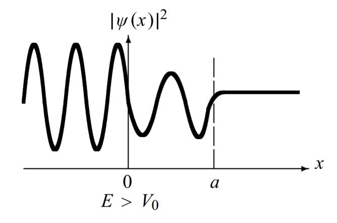
The constants B, C, D, and E can be obtained in terms of A from the boundary conditions:  $\psi(x)$  and  $d\psi/dx$  must be continuous at x = 0 and x = a, respectively:
