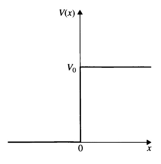
Classically, the particles arriving at the potential step from the left (with momenta  $p = \sqrt{2mE}$ ) will come to a stop at x = 0 and then all will bounce back to the left with the magnitudes of their momenta unchanged. None of the particles will make it into the right side of the barrier x = 0; there is total reflection of the particles. So the motion of the particles is reversed by the potential barrier.
