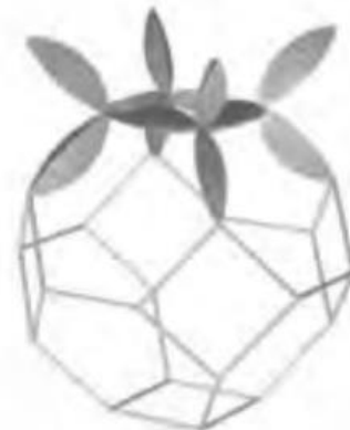
Figure 8.5. Fermi surface for three electrons per site in an fcc crystal. On the left the free-electron Fermi surface is shown in the extended zone scheme, while on the right the same surfaces are projected back into the first Brillouin zone in the reduced zone scheme.
