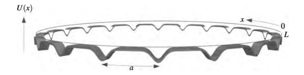
The setting for Bloch's theorem in one dimension is a potential U(x) of period *a* on a periodic domain of length *L*
