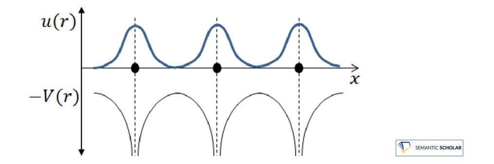
The periodic potential of a crystal results in a delocalized electron. The Bloch theorem requires the electronic wavefunction have the same periodicity as the lattice and therefore has a slowly varying envelope u(r).
