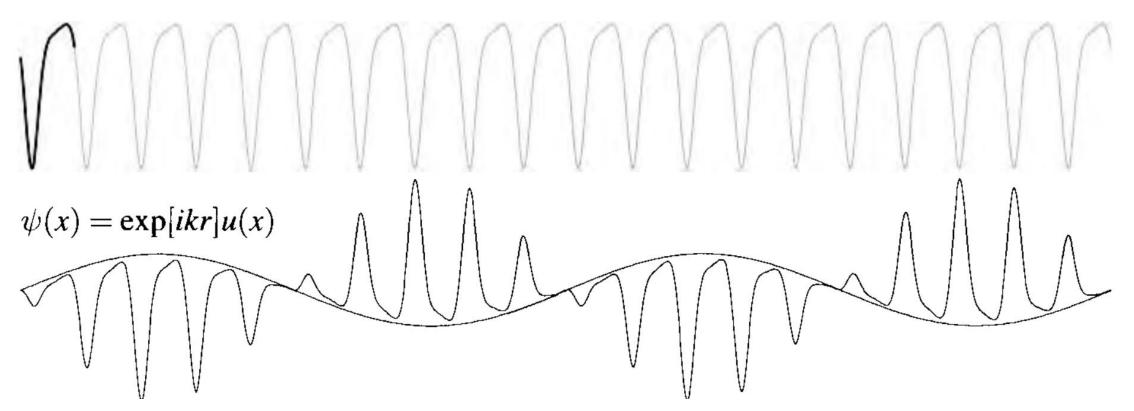
Bloch wave functions are periodic functions u(r) modulated by a plane wave of longer period. The lower portion of the figure displays the real part of  $\psi(x)$
